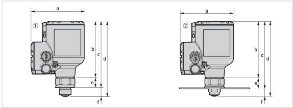
Figure 2-16: DN25 / 1" Lens antenna versions
