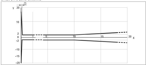
Figure 2-1: DN20  $(\frac{3}{4})$  Lens antenna: measuring accuracy (graph of measuring accuracy in mm against measuring distance in m)
