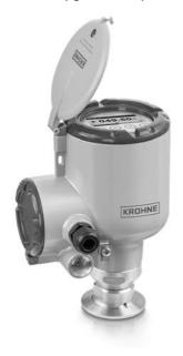
This 80 GHz FMCW radar transmitter for hygienic liquid applications in the pharmaceutical, food and beverage industries is CIP-SIP suitable and offers a large choice of hygienic process connections: Tri-Clamp®, Tuchenhagen VARIVENT®, SMS, DIN 11851, DIN 11864-1 Form A, NEUMO BioControl®.
