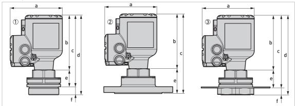
Figure 2-18: DN70 / 3" Lens antenna versions
