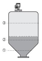
A strapping table function is available in the configuration menu for volume or mass measurement. Up to 50 volume (mass) values can be related to level values. For example:
