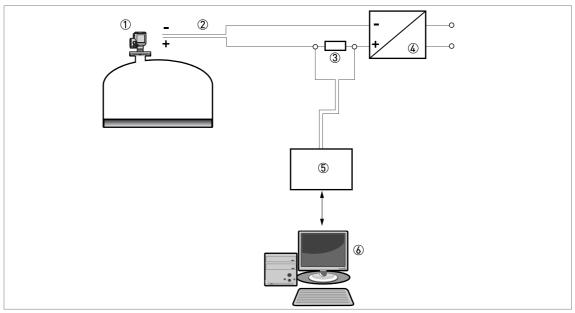
Figure 4-4: Point-to-point connection (non-Ex)
