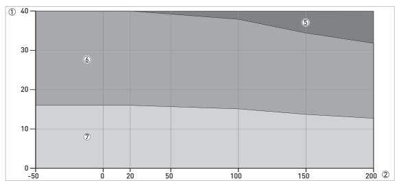
Figure 2-11: Pressure / temperature de-rating (EN 1092-1), flange and threaded connection, in °C and barg
