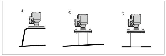
Figure 3-8: Device installation on tanks made of a non-conductive material
