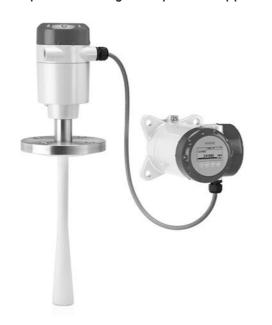
This 10 GHz 2-wire FMCW radar level transmitter measures distance, level, volume, mass and flow rate of liquids and pastes. It is ideal for corrosive products with its PP or PTFE antenna options. It features unique PP and PTFE antennas for aggressive products. The device is able to measure distances up 30 m / 98.4 ft in process conditions up to +250°C / +482°F and 40 barg / 580 psig.
