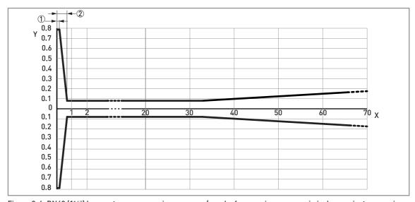
Figure 2-6: DN40 ( $1\frac{1}{2}$ ") Lens antenna: measuring accuracy (graph of measuring accuracy in inches against measuring distance in ft)
