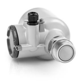
The small beam angle and negligible dead zone of this 80 GHz FMCW radar level transmitter makes it the premium choice for liquids in small and narrow tanks with internal obstructions like agitators or heating coils, as well as tanks with long nozzles. It can even measure through tank roofs made of non-conductive material (e.g. plastic, fiberglass or glass). The flush-mounted PEEK Lens antenna (no tank intrusion) is insensitive to deposit.
