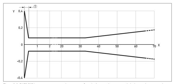
Figure 2-8: DN70 (3") Lens antenna: measuring accuracy (graph of measuring accuracy in inches against measuring distance in ft)
